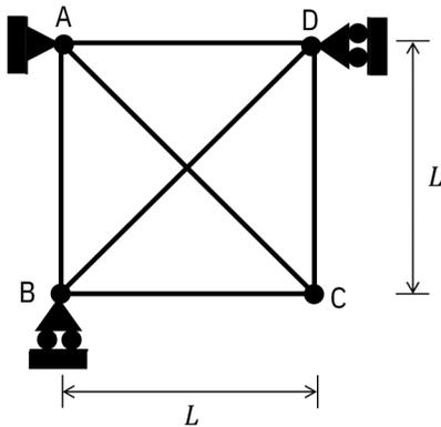
Structure II: Pin-jointed truss, with hinge support at A, and rollers at B and D
