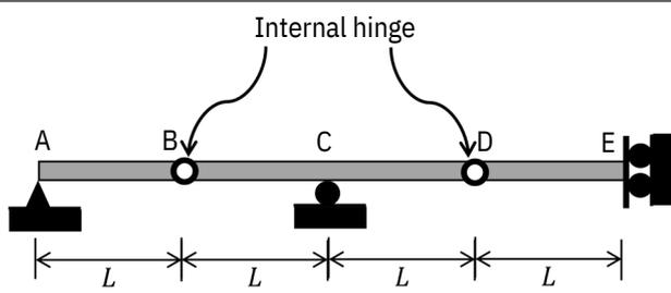
Structure I: Beam with hinge support at A, roller at C, guided roller at E, and internal hinges at B and D
