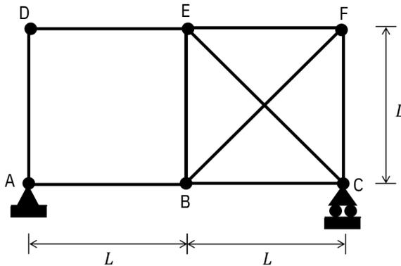
Structure III: Pin-jointed truss, with hinge support at A and roller at C
