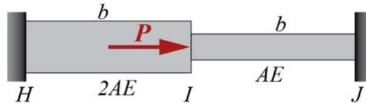
To make the axial force in rod HI equal to zero, the value of the external force  $P$  (in N) is \_\_\_\_\_. (round off to the nearest integer)
