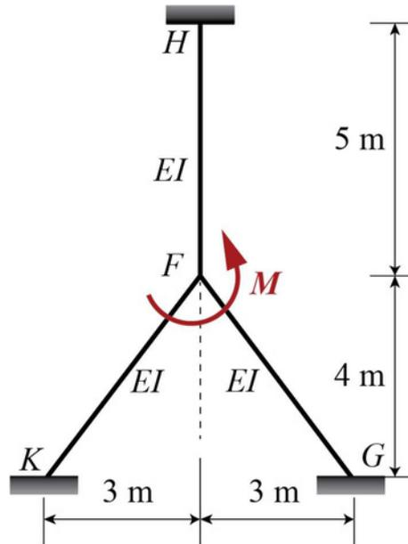
If the magnitude (absolute value) of the support moment at H is 10 kN-m, the magnitude (absolute value) of the applied moment  $M$  (in kN-m) to maintain static equilibrium is \_\_\_\_\_. (round off to the nearest integer)
