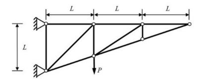
Neglecting self-weight of the members, the number of zero-force members in the truss under the action of the load P, is
