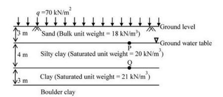
Immediately after preloading, the effective stresses (in kPa) at points P and Q, respectively, are
