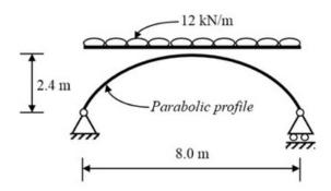
Neglecting self-weight, the maximum bending moment generated in the structure (in kN.m, round off to the nearest integer), is \_\_\_\_\_\_.
