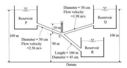
Considering head loss only due to friction (with friction factor of 0.03 for all the pipes), the height of water level in the lowermost reservoir R (in m, round off to one decimal place) with respect to the datum, is \_\_\_\_\_\_.
