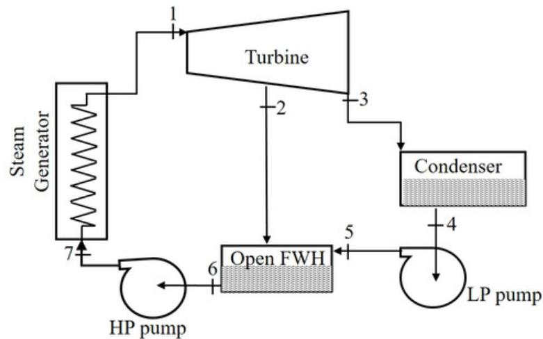
Specific enthalpy of steam at location 2 is  $2624$  kJ/kg, specific enthalpy of water at location 5 is  $226.7$  kJ/kg and specific enthalpy of saturated water at location 6 is  $708.6$  kJ/kg. If the mass flow rate of water entering the open feed water heater (at location 5) is  $100$  kg/s then the mass flow rate of steam at location 2 will be \_\_\_\_\_ kg/s (round off to one decimal place).
