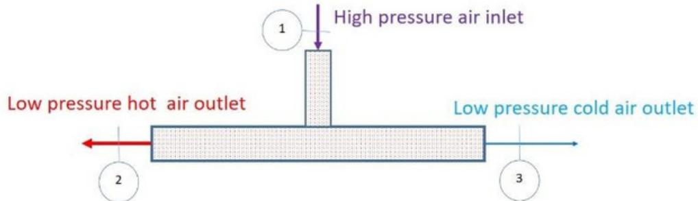
Assume constant specific heat of air is 1005 J/kg.K and gas constant is 287 J/kg.K. There is no work transfer across the boundary of this device. The rate of entropy generation is \_\_\_\_\_ kW/K (round off to one decimal place).
