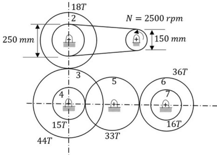
Diameters of pulleys of belt drive and number of teeth ( $T$ ) on the gears 2 to 7 are indicated in the figure. The speed and direction of rotation of gear 7, respectively, are
