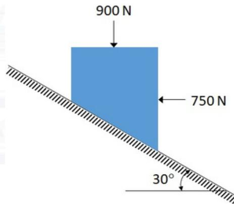
The coefficient of static friction between the block and surface is \_\_\_\_\_ (round off to two decimal places).
