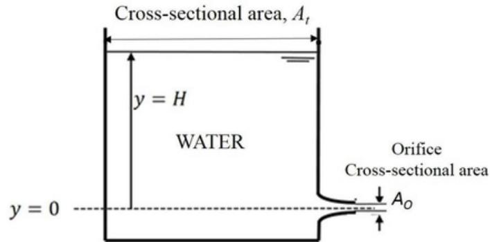
Neglecting any losses, the time taken by water in the tank to reach a level of  $y=H/4$  is \_\_\_\_\_ seconds (round off to one decimal place).
