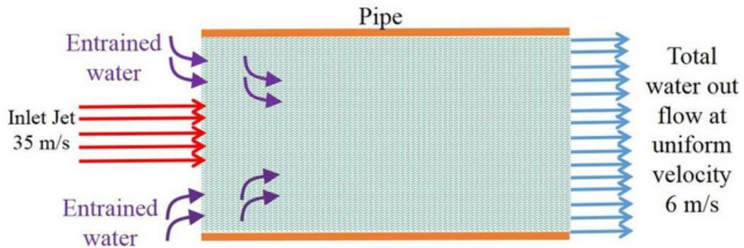
The flow rate of entrained water is \_\_\_\_\_ litres/s ( round off to two decimal places).
