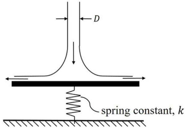
If the spring shows a steady deflection of  $1 \text{ cm}$  upon impingement of jet, then the velocity of the incoming jet is \_\_\_\_\_  $\text{m/s}$  (round off to one decimal place).
