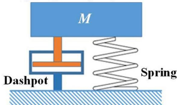
If the amplitude of the free vibration response reduces from  $8 \text{ mm}$  to  $1.5 \text{ mm}$  in 3 cycles, the damping ratio of the system is \_\_\_\_\_ (round off to three decimal places).
