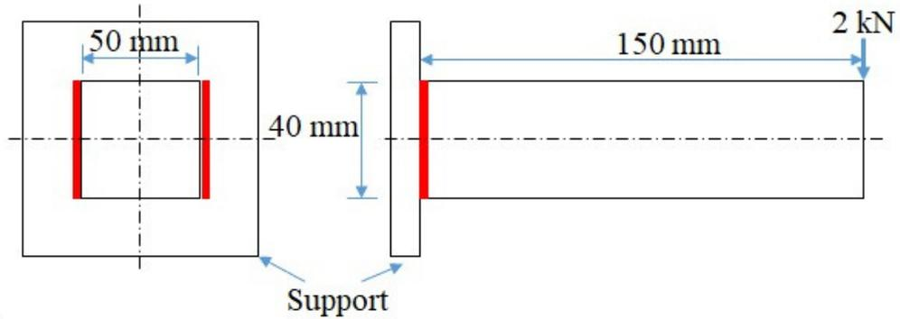
Considering that the allowable shear stress in weld is  $60 \text{ N/mm}^2$ , the minimum size (leg) of the weld required is \_\_\_\_\_ mm (round off to one decimal place).
