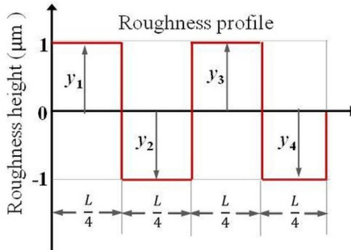
The center line average roughness  $R_a$ , in  $\mu\text{m}$ ) of the measured length ( $L$ ) is
