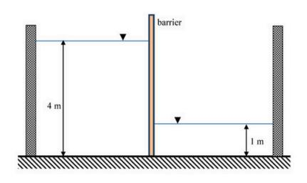
Taking the density of water as  $1000 \text{ kg/m}^3$ , and the acceleration due to gravity as  $10 \text{ m/s}^2$ , the maximum absolute bending moment developed in the cantilever is kN-m (round off to the nearest integer).
