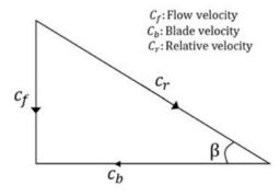
The diameter at this section is 3 m. The hub and tip diameters of the blade are 2 m and 4 m, respectively. The water volume flow rate is 100 m<sup>3</sup>/s. The rotational speed of the turbine is 300 rpm. The blade outlet angle  $\beta$  is \_\_\_\_\_\_ degrees (round off to one decimal place).
