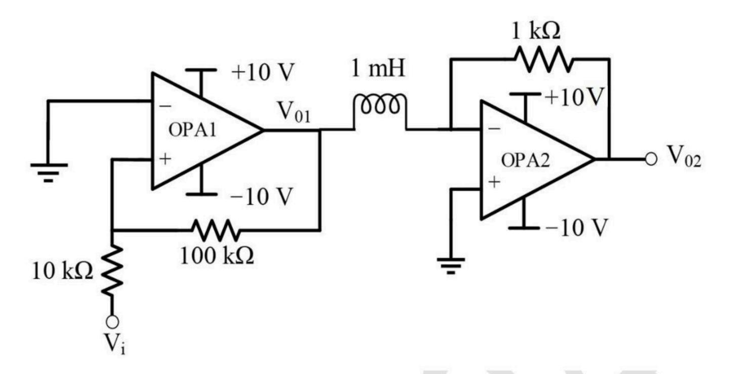
Assume that the initial inductor current is 0 A. The input voltage ( $V_i$ ) is a triangular signal with peak voltages of  $\pm 2$  V and time period of 8  $\mu$ s. Which one of the following statements is true?
