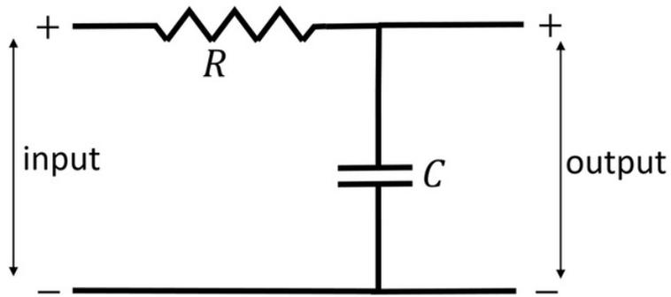
(A)  $R = 1 \text{ k}\Omega, C = 0.1 \text{ }\mu\text{F}$
