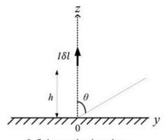
Infinite conducting plane
